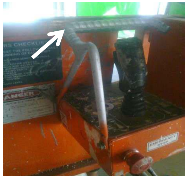
Fig 1: Unauthorised 'Adhoc' guard (arrowed) welded above Manufacturers original guard may cause scissor lift to become unstable if hoses, leads etc. become snagged on it.
